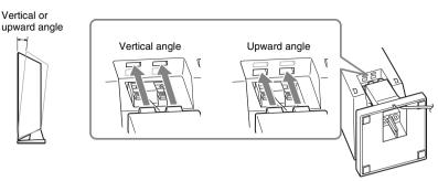
4 Thread the speaker cord though the slit of the stand base to prevent the cord from being twisted or pinched.
